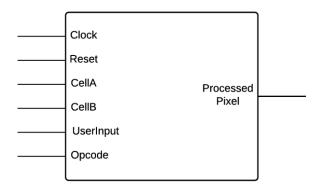
Figure 1: Cell Processor Block Diagram
