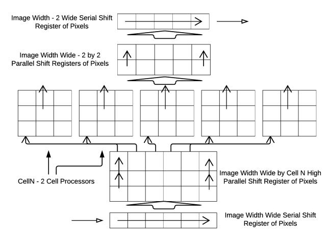
**Figure 4: Image Processor Architecure**
